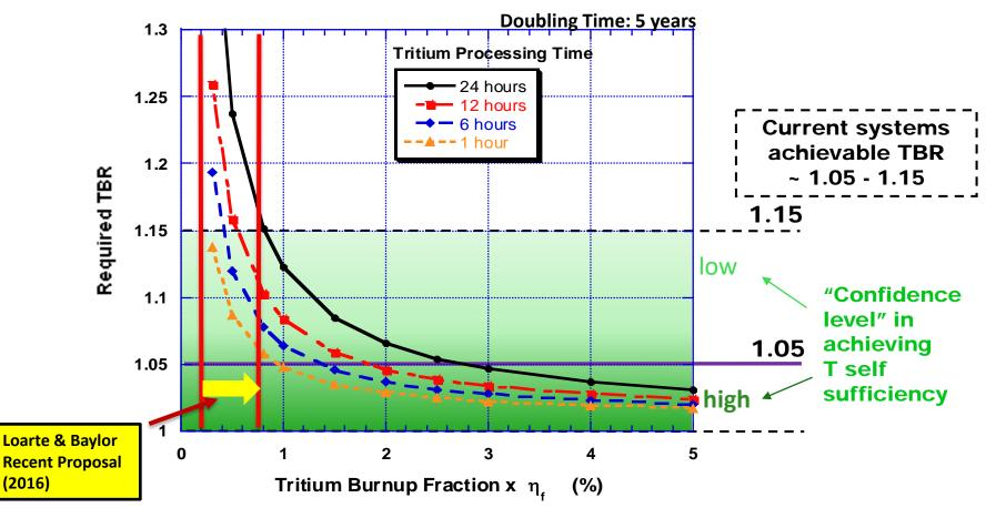
State of the art (ITER:  $f_b \sim 0.35\%$ ,  $\eta_f < 50\%$ ) achieving T self-sufficiency is <u>Unlikely</u>.
