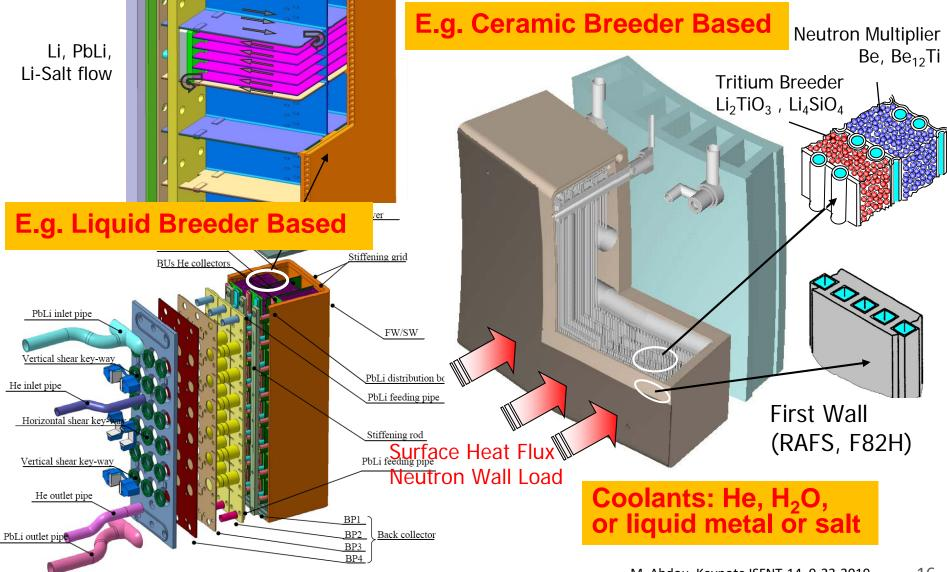
For 30 years fusion researchers studied Liquid Metal MHD Flow Behavior in Blankets as if it were PURELY in the Presence of Magnetic Field (i.e. separate effect). So, the common assumption has been:
