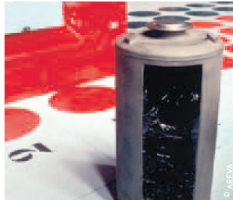
Figure 2 – Vitrified high-level metallic waste container
