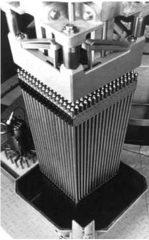
Figure 1.1: PWR fuel assembly (left) and CANDU fuel bundle (right). A typical PWR assembly is made up of 1 cm diameter fuel pellets inside zircaloy tubes. The assembly is approximately 4 m in length and 20
