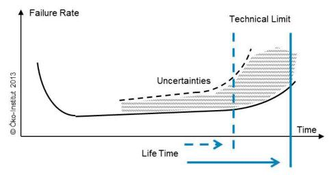
Figure 1.9 – Schematic 'bathtub curve' diagram of failure rate.
